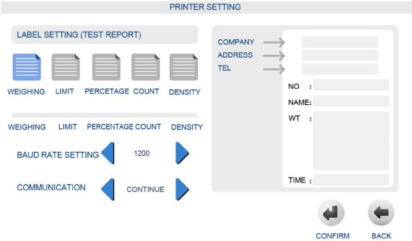
We can choose the suitable baud rate and communication style for different print or connect with the computer.
