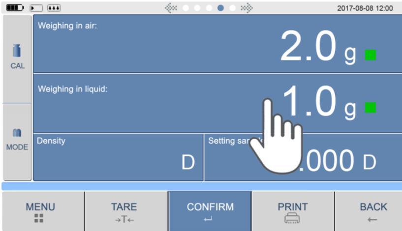
Step 4: Press the density, the result will be come out, the density unit is  $\text{g/cm}^3$
