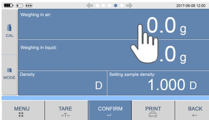
When the weighing digit value stable, press again then will be show green square. Means confirm the weight in the air.
