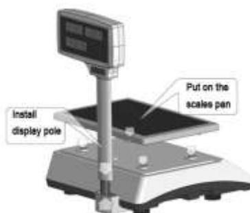
3. Turn on the power, then the scale will initialize. The display will show 0 after the initialize process, and a buzzer sound. And you can use the scales freely. If the display is not show 0, please press the ZERO key.
